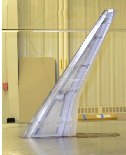
Fig. 1.3 CRM65 semi-span wind tunnel model tested at the University of Illinois.
